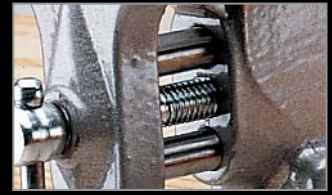
DOUBLE STEEL GUIDE BARS
